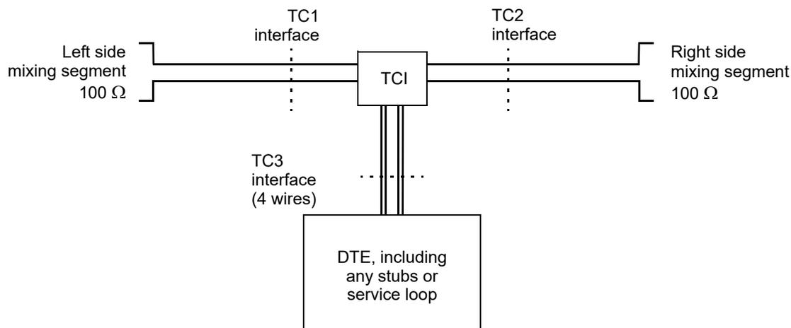
**Figure 168–22—TCI ports and connections**
