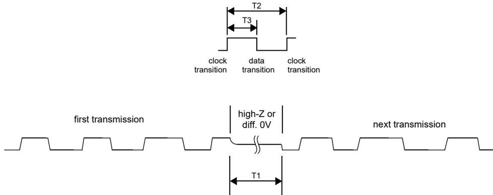
**Figure 168–14—DME encoding scheme**
