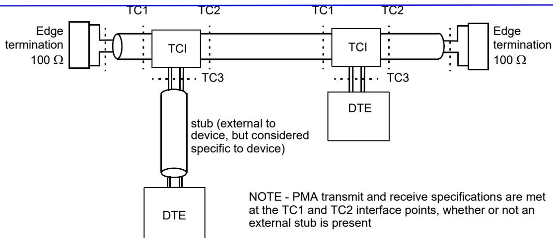
**Figure 168–21—Mixing segment and reference points**
