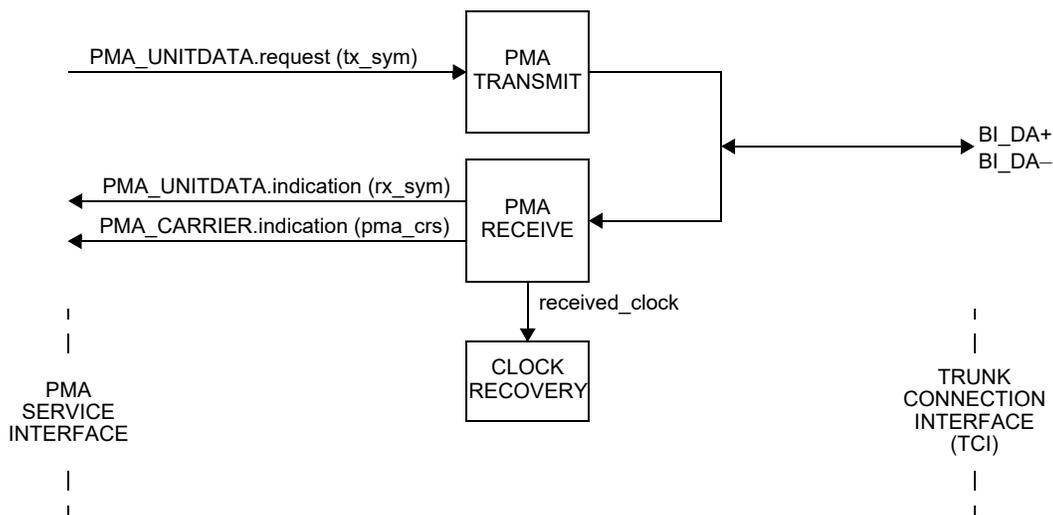
Figure 168–13—PMA functional block diagram
