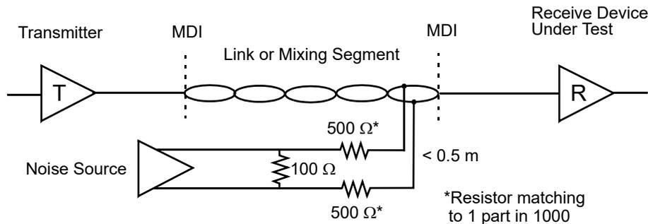
Figure 168–19—Alien crosstalk noise rejection test set-up
