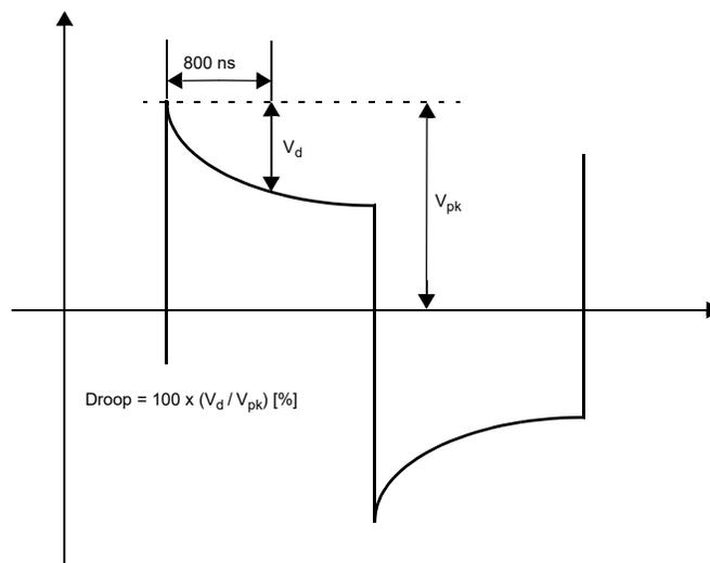
Figure 168–17—Transmitter output droop
